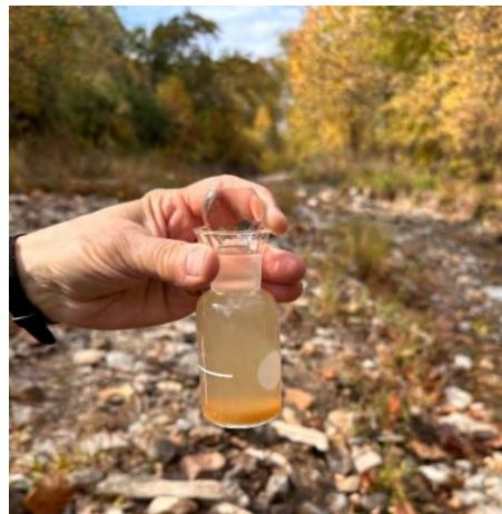
Dissolved Oxygen is measured with a colorimetric assay
